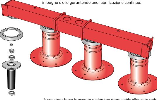
A constant force is used to action the drums; this allows to reduce the wear of the gears and the transmission shaft that is inside the tank. The bevel gears rotate in an oil bath ensuring continuous lubrication.
