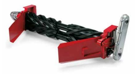
To accelerate the drying process and produce optimal quality fodder, the mowers can be provided with a conditioner with helical rubber rollers (Chevron type), where both the rollers are drive rollers due to the dual transmission. This eliminates the risk of clogging. The conditioner is self-cleaning with closed box
